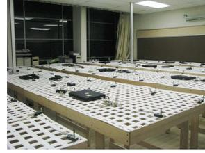
Figure 3. *NetEye* wireless sensor network testbed
